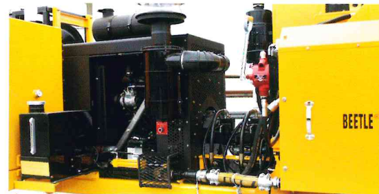
A PowerTech Plus 4045H engine hydraulically powers the new Gill Beetle 300.
